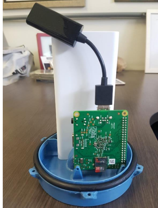
Fig. 2 – Waterproof housing (inside)
