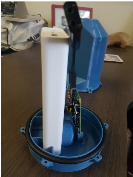
Fig. 3 – Waterproof housing (fitting for the recorder components)
